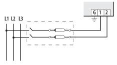
Line to Line from 90 VAC to 600 VAC (UL) (520 VAC for CE). In UL installations the lines may be floating (such as a delta). If any lines are tied to an earth (such as a corner grounded delta), see the Line to Neutral installation limits. In CE compliant installations, the lines must be neutral (earth) referenced at less than 300 VAC, "
