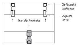
3. To reduce horizontal shifting across the DIN rail, use two Veris AVO2 end stop clips.
