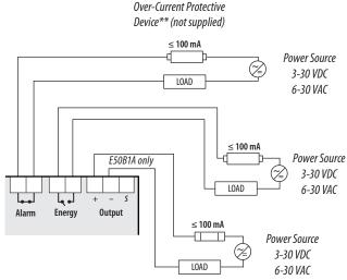
The solid state pulse outputs are rated for 30VAC/DC nom.
