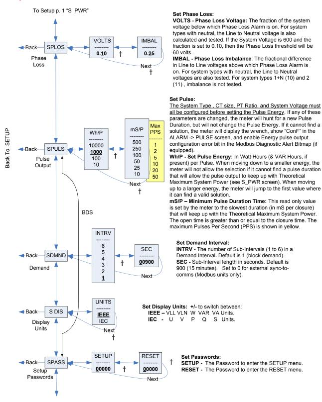
† When leaving this parameter screen using the right button ( ), the display will briefly indicate "SAvEd)" to confirm that any changes made have been accepted.
