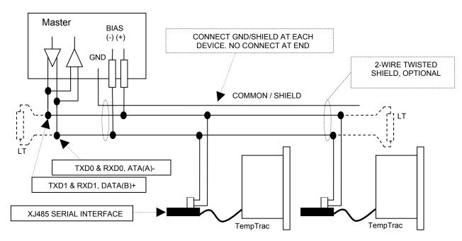
*Figure 3* Wiring of a typical Modbus RTU network with TempTrac<sup>®</sup> devices
