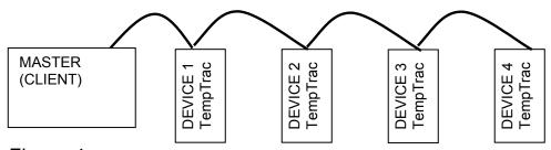
Figure 4 Correctly wired RS-485 Daisy Chain
