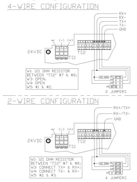
Note: W1 jumper should only be inserted in the last meter in the RS485 daisy chain
