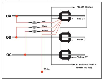
Figure 4 Typical 480 Vac max., 3Ø, 3-wire installation
