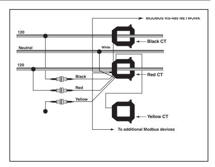
Figure 5 Typical 240/120 VAC 1Ø, 3-wire installation
