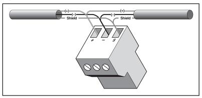
Figure 8 Wiring the RS-485 terminal block
