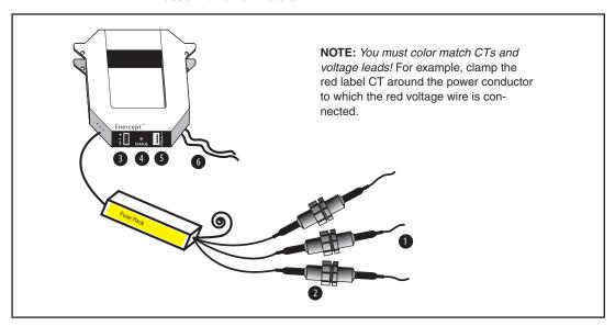
Figure 1 Diagram of typical Enercept meter
