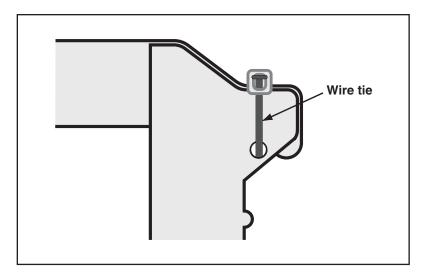
Figure 7 Wire tie used to secure I-Bar
