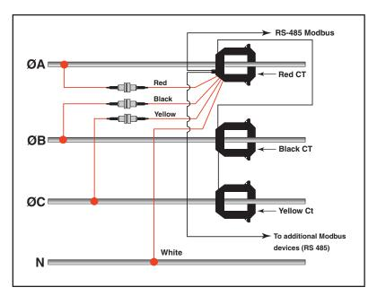
Figure 3 Typical 480 Vac max., 3Ø, 4-wire installation
