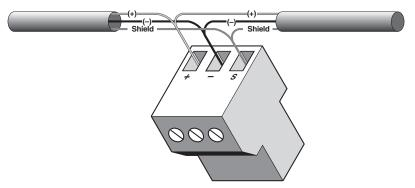
Figure 12 Connecting communications wires to the RS-485 terminal block.
