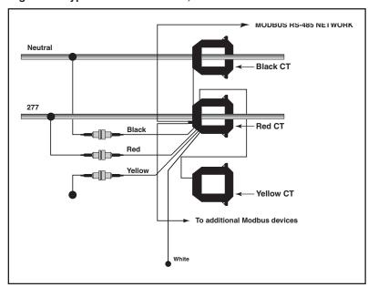
Figure 6 Typical 277 VAC 1Ø, 2-wire installation
