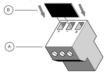
Figure 13 Installing the MCTAS-485 terminator.
