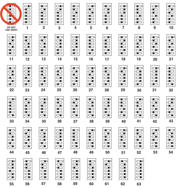
Figure 2 Address selection switches
