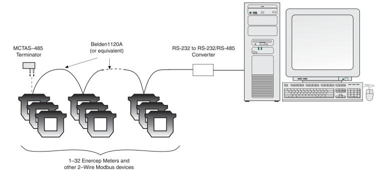
Figure 10 Enercept meters connected to a PC's serial port.
