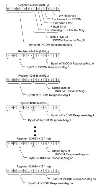
Figure 12: Pass-Through Response Data Format
