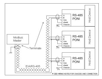
Figure 9. Typical RS-485 PONI Wiring Diagram
