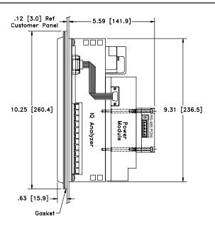
Figure2: Mounting to an IQ Analyzer
