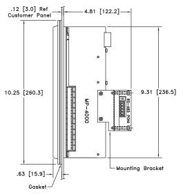
Figure 6: Mounting to an MP-4000
