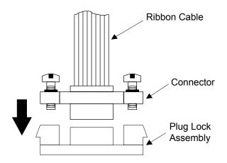
Figure 3: Attaching the Cable to the Plug Lock Assembly
