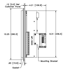
Figure 5: Mounting to an MP-3000
