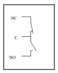
FIGURE 2–1: Internal Schematic (De-energized State)
