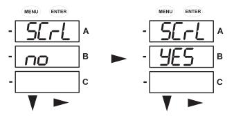
FIGURE 7-4: Scroll Mode Configuration
