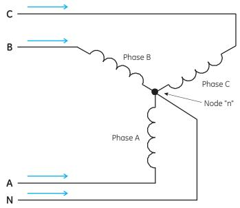
FIGURE 1–6: Three-Phase Load Illustrating Kirchhoff's Law and Blondell's Theorem
