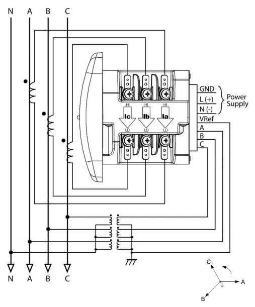
FIGURE 4–7: 4-Wire Wye with 3 PTs and 3 CTs, 3 Element
