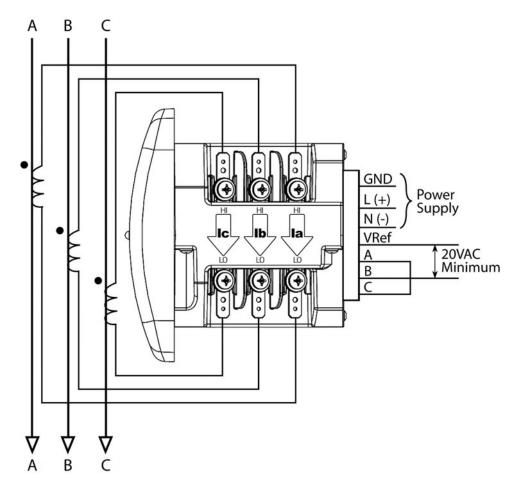
FIGURE 4–12: Current-Only Measurement (Three-Phase)
