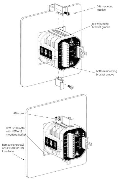
FIGURE 3-3: DIN Mounting Procedure
