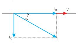
FIGURE 1-9: Voltage and Complex Current
