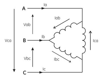
FIGURE 1–3: Three-phase Delta Winding Relationship
