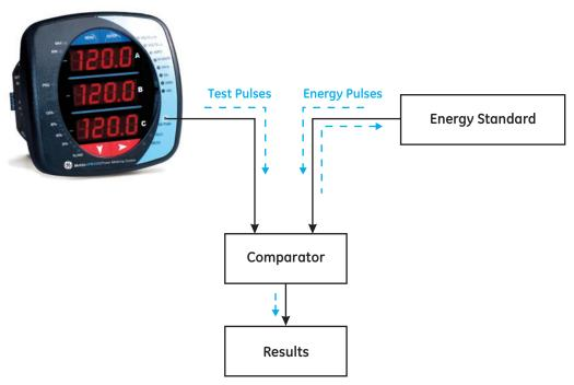
FIGURE 6-4: Using the Watt-Hour Test Pulse
