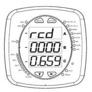
FIGURE 7–2: Typical Wh Reading
