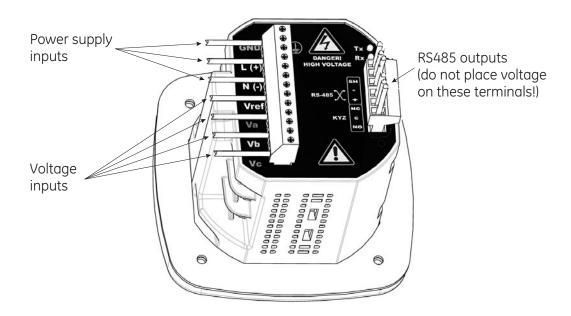
FIGURE 4-4: Voltage Connection
