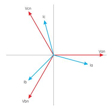
FIGURE 1-2: Three-phase Voltage and Current Phasors for Wye Winding
