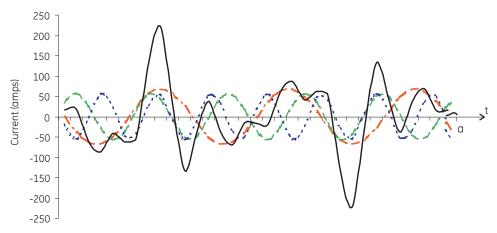
FIGURE 1-12: Waveforms of the harmonics
