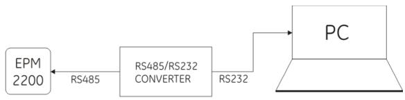
FIGURE 5–2: EPM2200 Connected to PC via RS485
