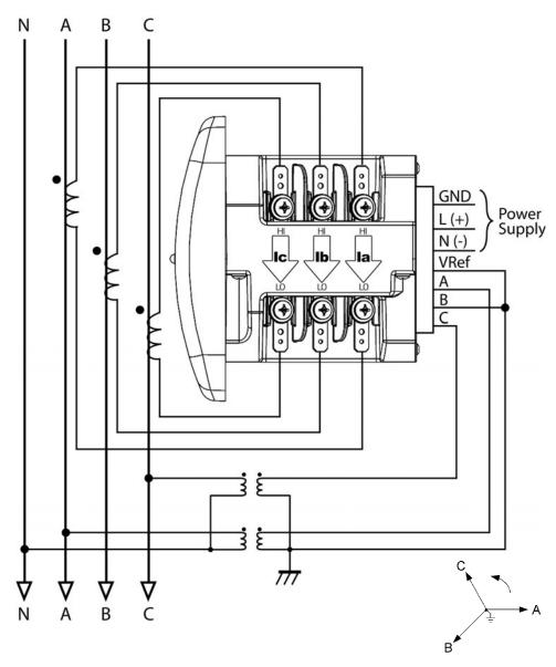
FIGURE 4-8: 4-Wire Wye with 2 PTs and 3 CTs, 2.5 Element
