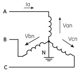
FIGURE 1-1: Three-phase Wye winding
