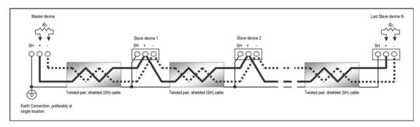
FIGURE 5-4: RS485 Daisy Chain Connection
