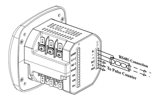
FIGURE 5-1: 485P Option with RS-485 Communication Installation
