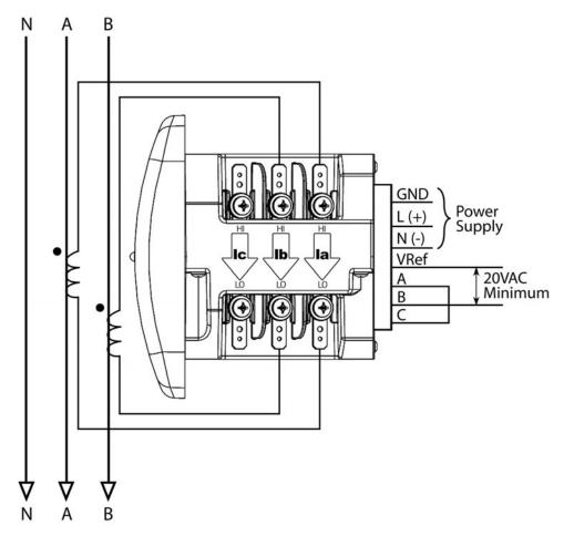
FIGURE 4–13: Current-Only Measurement (Dual-Phase)
