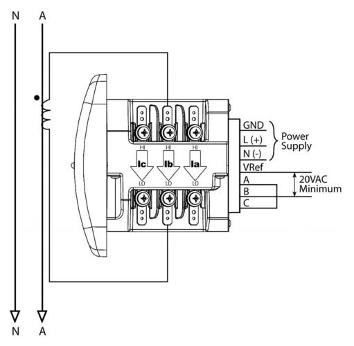
FIGURE 4–14: Current-Only Measurement (Single-Phase)
