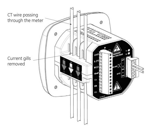
FIGURE 4–2: Pass-Through Wire Electrical Connection
