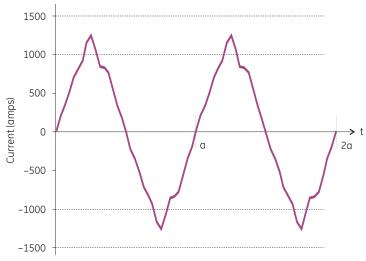
FIGURE 1-11: Distorted current wave
