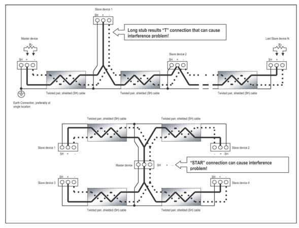
FIGURE 5-5: Incorrect "T" and "Star" Topologies
