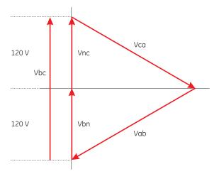
FIGURE 1–5: Three-Phase, Four-Wire Delta Phasors
