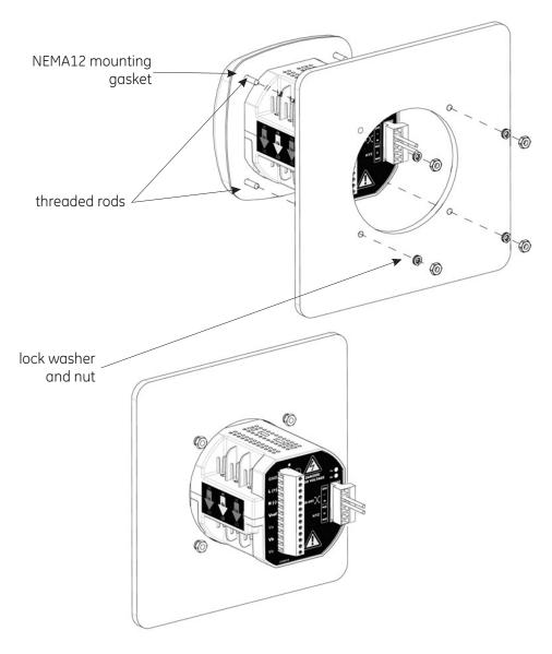
FIGURE 3-2: ANSI Mounting Procedure
