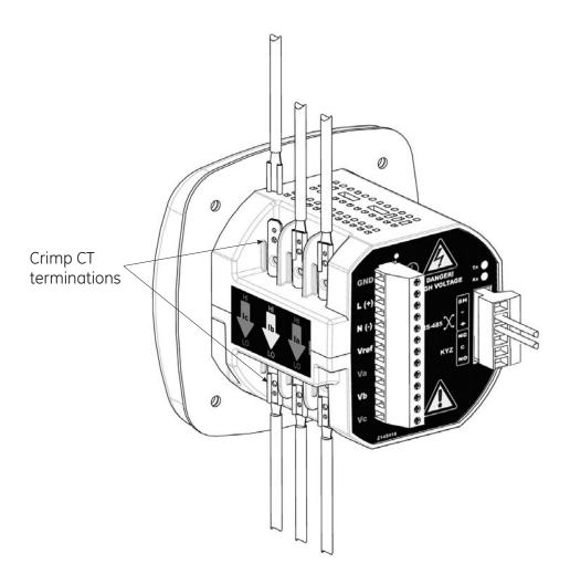
FIGURE 4–3: Quick Connect Electrical Connection
