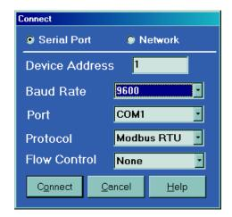
FIGURE 5-7: Serial Port settings
