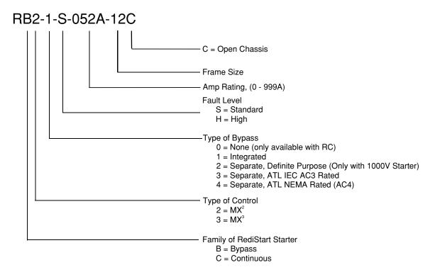
Example of Model Number: RX2-1S-361A-14C A RediStart starter with bypass,  $MX^2$  control, Integrated Bypass, Standard Fault, 361 Amp unit, Frame 14, open Chassis.
