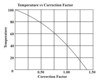
Example: If a motor operates at  $0^{\circ}$ C, then a 1.36 correction factor could be applied to the overload multiplier. This could give a theoretical overload multiplier of 1.36 x 1.25 or 1.70. The highest legal NEC approved value of overload multiplier is 1.40, so this could be used.
