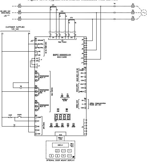
Figure 43: A Typical ATL Starter Schematic with the MX<sup>2</sup>
