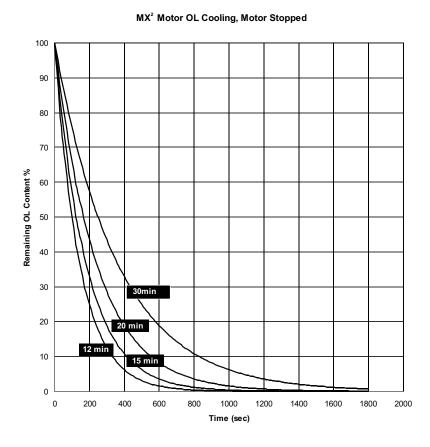
If the motor manufacturer does not specify the motor cooling time, the following approximations for standard TEFC cast iron motors based on frame size can be used:
