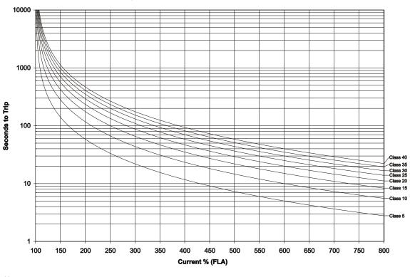
Figure 25: Commonly Used Overload Curves
