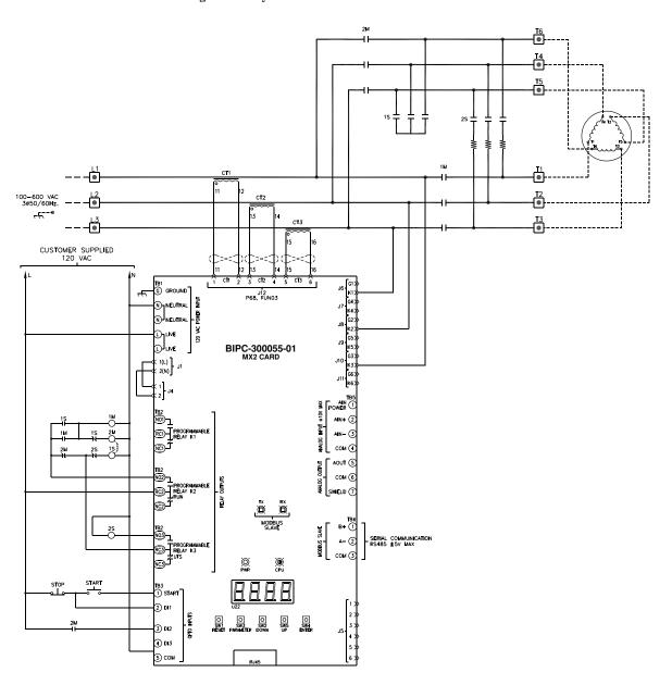
The MX<sup>2</sup> utilizes an intelligent Wye to Delta transition algorithm. During starting, if the measured motor current drops below 85% of FLA and more than 25% of the Up To Speed timer setting has elapsed, then a Wye to Delta transition occurs. The intelligent transition algorithm prevents unnecessarily long motor starts which reduces motor heating. If a Wye to Delta transition has not already occurred, a transition always occurs when the complete Up To Speed Time expires.
