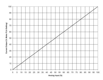
A reference input value of 0% results in no output. A reference input value of 100% results in a current output equal to the Motor FLA setting. The actual voltage or current input that results in a given output can be adjusted through the use of the Analog Input Offset and Analog Input Span parameters.
