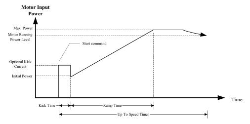
Power control acceleration can be very useful for a variety of applications. Power control generally should not be used in applications where the starting load varies greatly during the start such as with a reciprocating compressor. Power control is not recommended for starting of AC synchronous motors.
