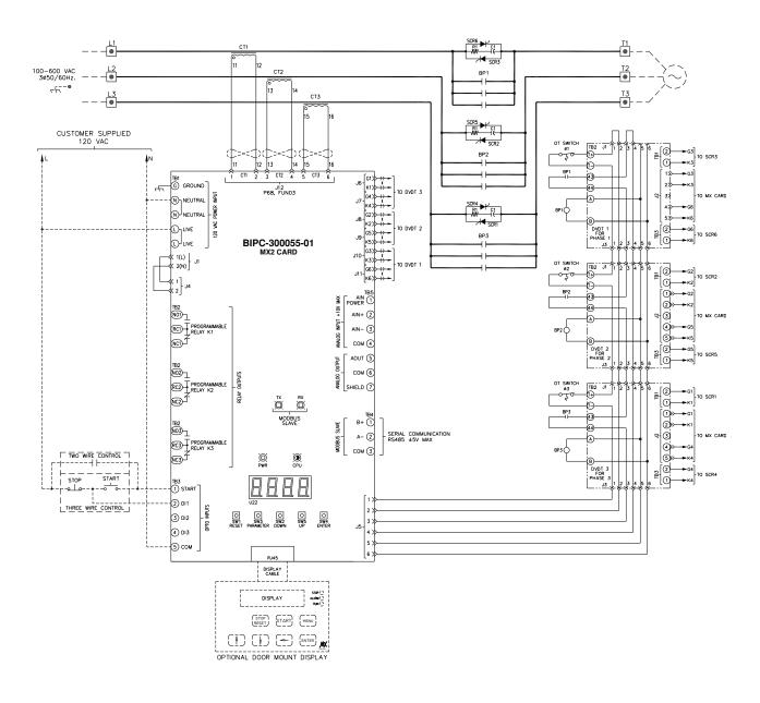
Figure 9: Power Schematic for RB2 High HP
