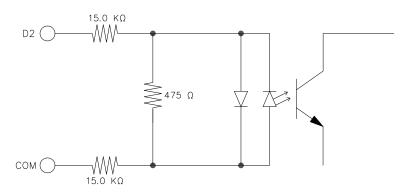
Figure 49: Analog Input Simplified Schematic
