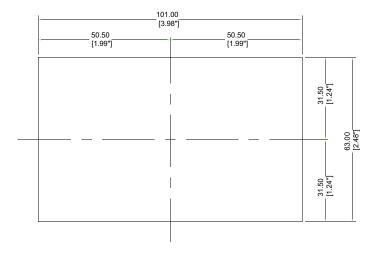
Figure 20: Large Display Keypad Mounting Dimensions Part # : KPMX3LLCD
