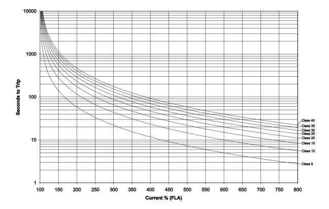
Figure 2: Commonly Used Overload Curves
