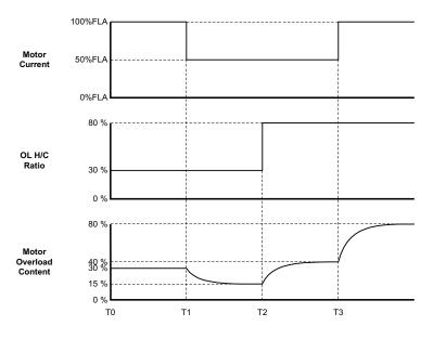
Figure 27: Motor Overload H© Ratio Example
