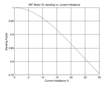
Figure 26: Overload Derating for Current Imbalance
