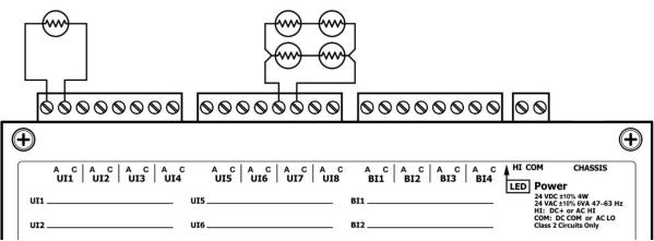
10 k $\Omega$  or 20k $\Omega$   $\,$  Type II or Type III Thermistors
