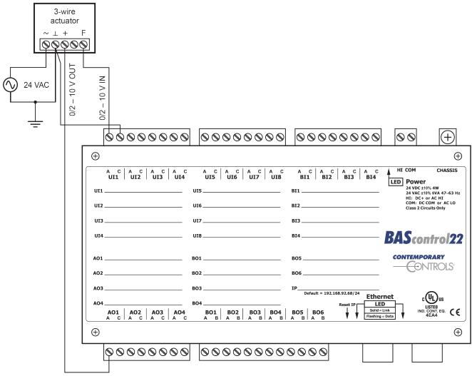
Figure 8 — Analog Output Connections
