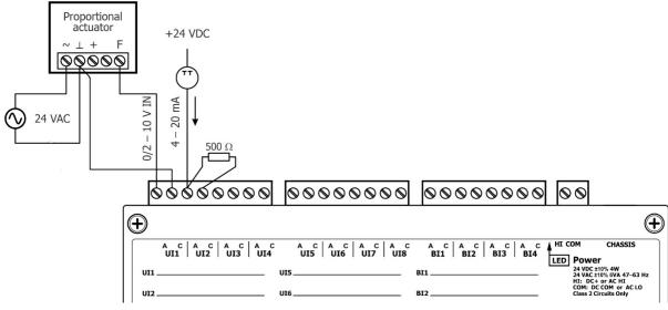
Figure 4 — Analog Input Connections
