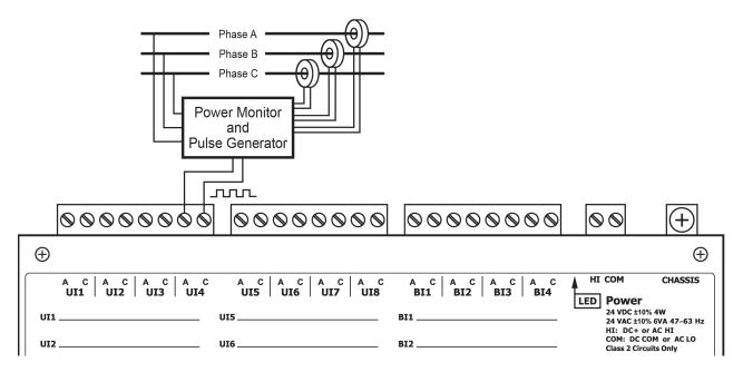
Figure 7 — Pulse Input Connections
