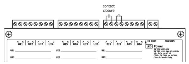
Figure 10 — Binary Input Connection
