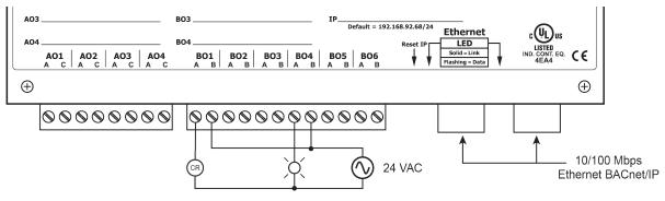
Figure 9 — Binary Output Connections
