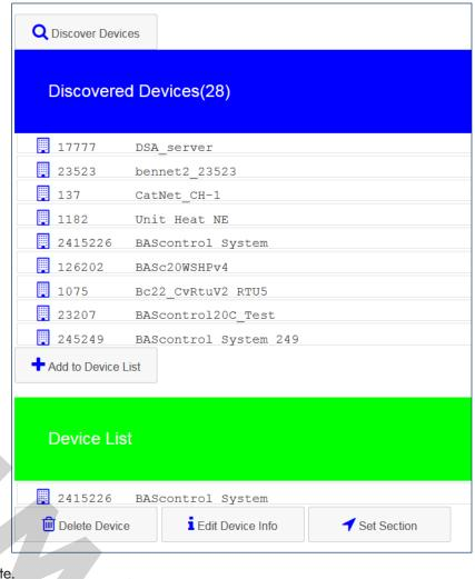
The BASintegrator is not only a head-end, it can also be used to help integrate systems for other head-ends. For example, the BASintegrator has its own internal points. These can be written or read from another head-end. These can also be used to help get data between networks with the BASintegrator binding feature. You can select a source point on network A and a destination point on network B and when the source point value changes, the destination point receives this
