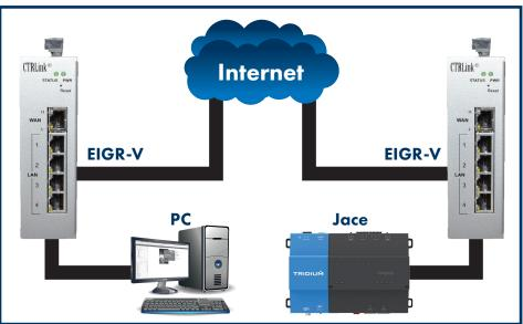
Scenario 6: Secure BACnet/IP communications between Jace and MS/TP devices.
