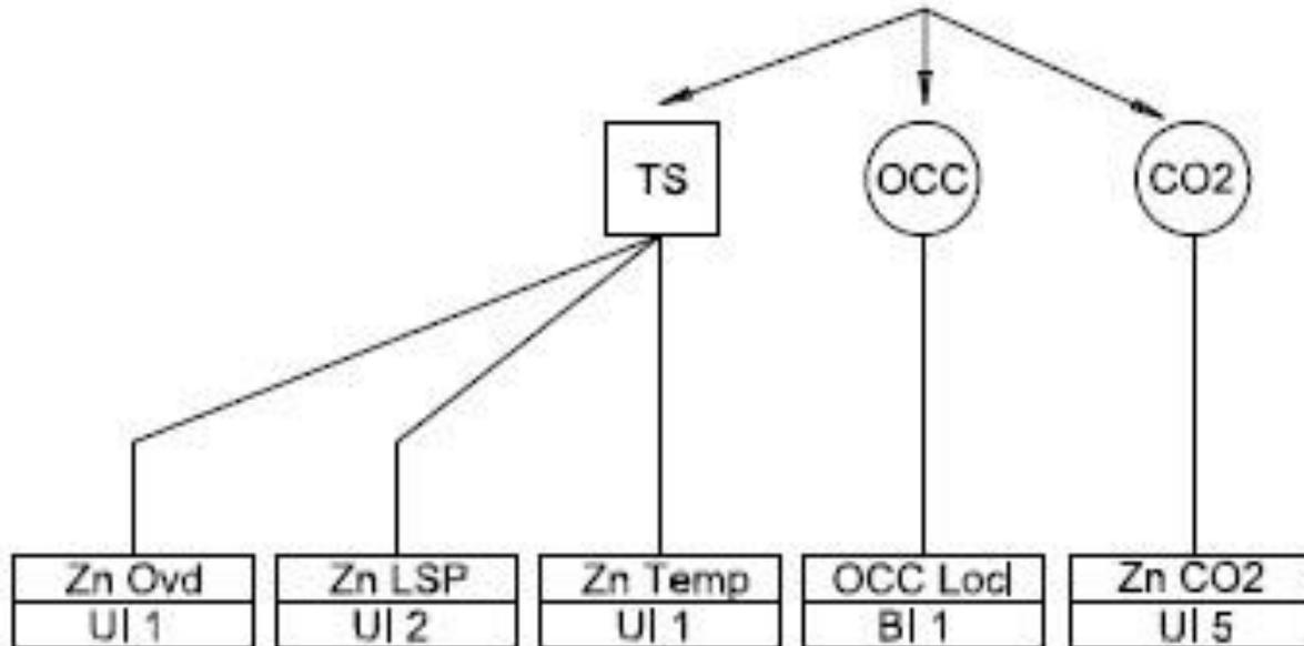
*A wall setter is optional. If no slider switch (ZnLSP) is discovered for setpoint control, then the program assumes BACnet client control of the setpoint. However, a space temperature sensor (ZnTemp) is needed which could be located in the zone or in the return air duct. By momentarily shorting out the zone temperature sensor, a momentary occupied (ZnOvd) signal is created.*
