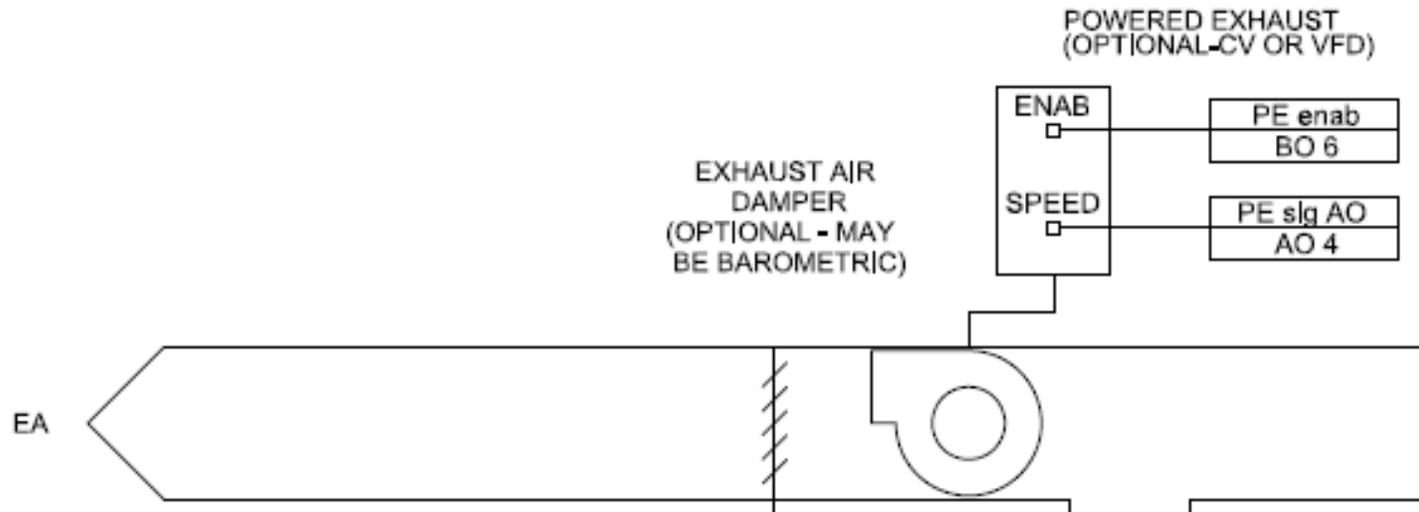
*For the exhaust duct, you can have a constant volume exhaust fan, a variable speed exhaust fan or no fan at all. The exhaust damper could be a simple barometric damper. Variable speed exhaust fan is based upon outside air damper position rather than building static pressure input.*
