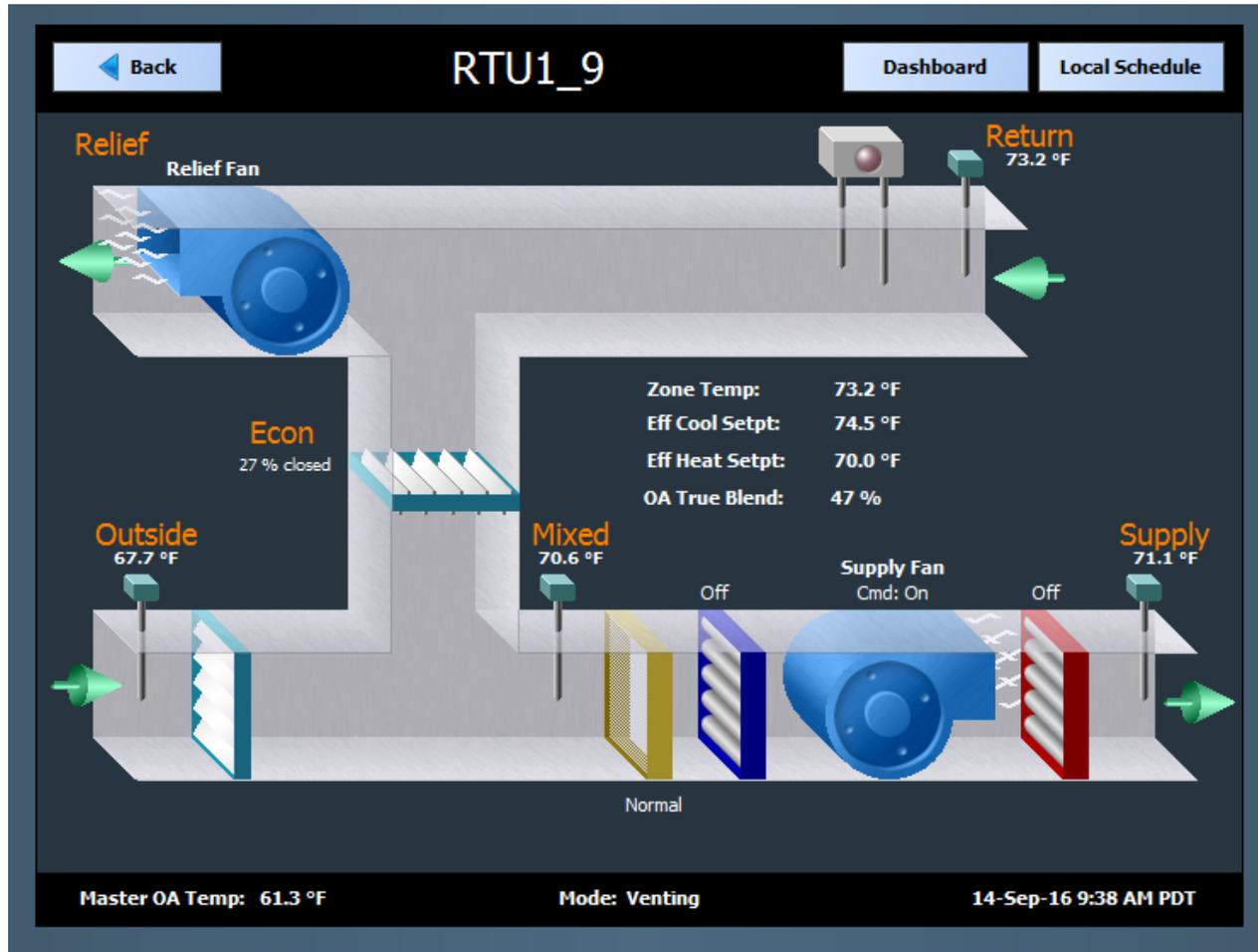
*The CvRTU series provides five pre-built control applications for rooftop units (RTUs) that will execute on a Contemporary Controls' BAScontrol22 BACnet/IP Sedona controller. Pre-built applications speed up installation time by only requiring configuration during installation.*
