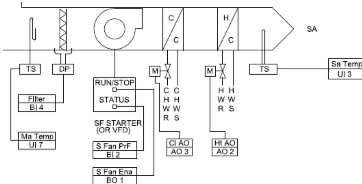
*It is also possible to have 0-10 volt analog control for chilled water (CHW) cooling and hot water (HW) heating. All other sensors remain the same as for staged heating and cooling.*
