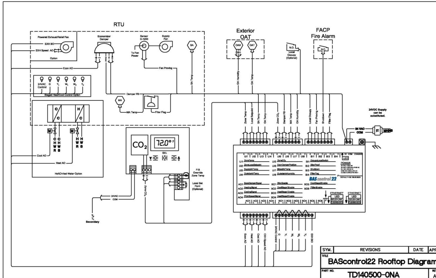
*To assist the panel builder in designing a panel, a sample wiring diagram is provided in .dxf format showing the interconnections between the controller and recommended ancillary equipment.*
