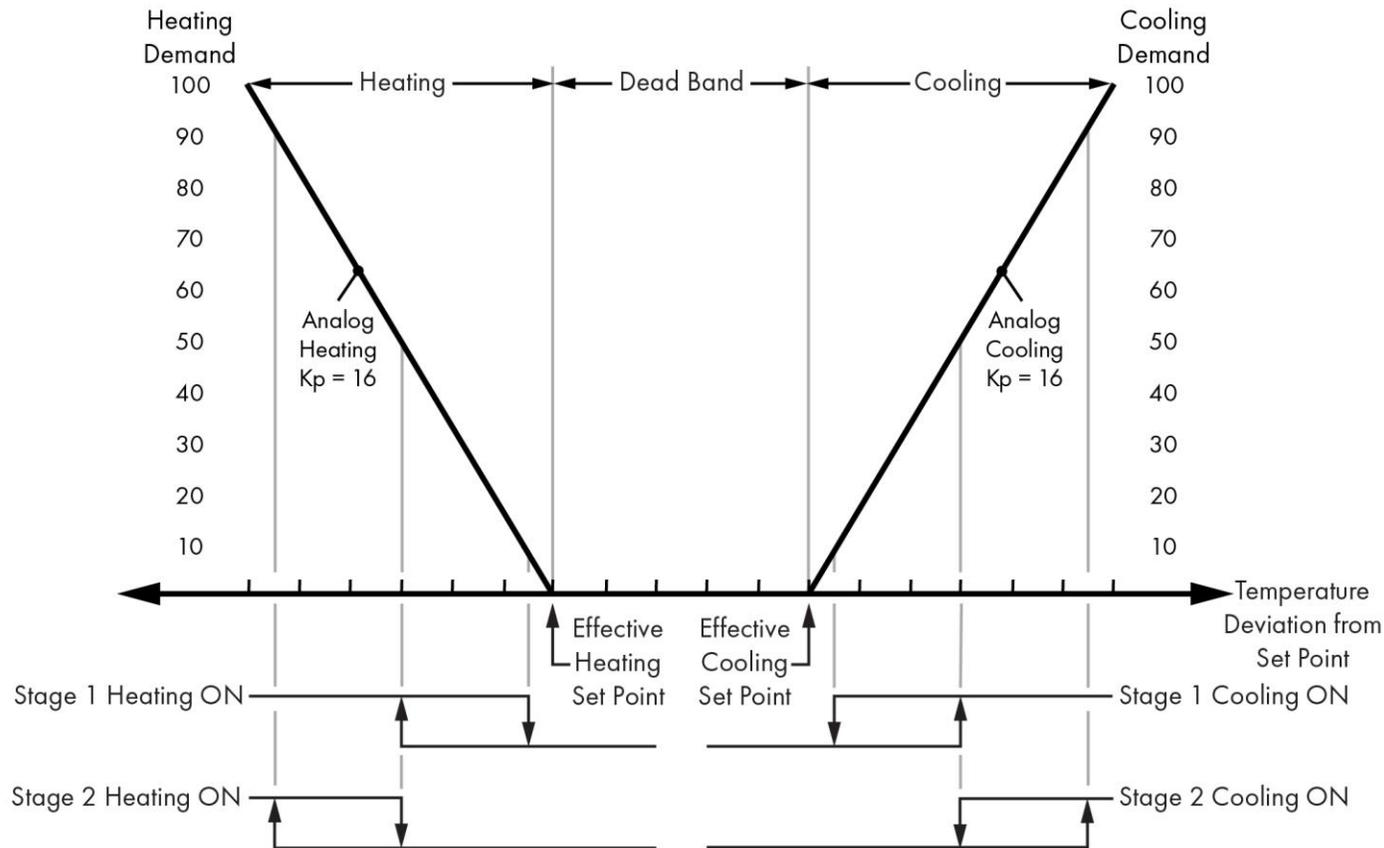
*Heating and cooling control utilize two enhanced PID components along with hysteresis and timer components. PID parameters can be changed as well as the hysteresis trip points and timer delays.*
