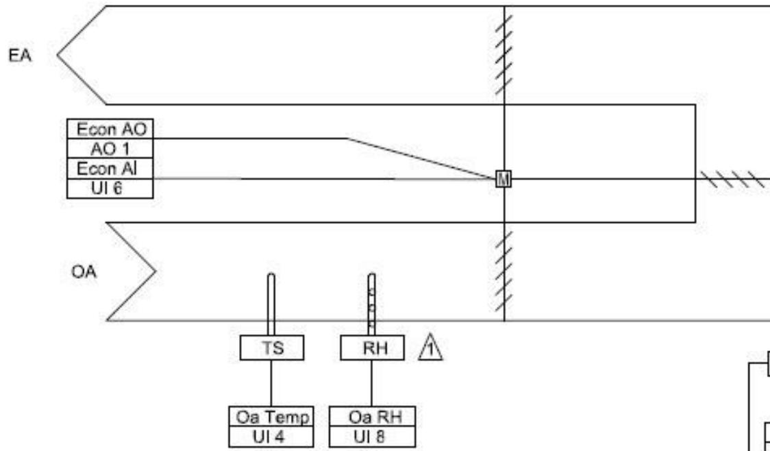
*You can also have a dry-bulb economizer requiring an outside air temperature sensor (TS), an enthalpy economizer requiring a relative humidity sensor (RH) in addition to the dry-bulb sensor or no economizer at all. A proportional damper actuator must be provided which has analog position feedback.*
