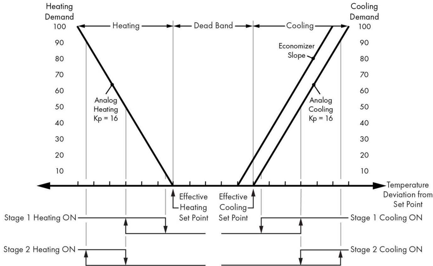
*Economizers add an early stage of free-cooling assuming the outside temperature (dry-bulb) or outside humidity (dry-bulb and relative humidity) are conducive to free-cooling. An additional PID component and other logic are used for economizing.*
