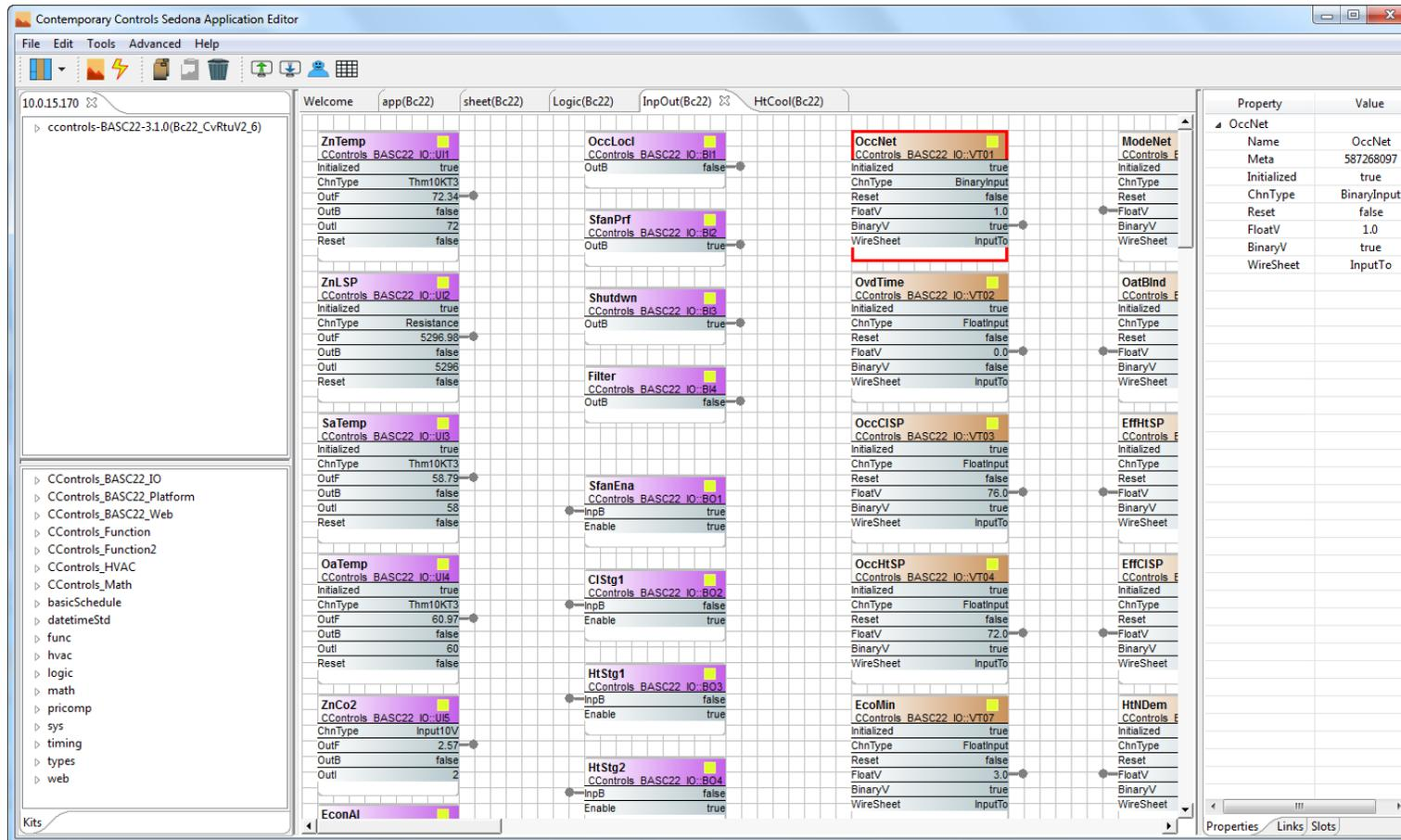
*All I/O points can be found in one folder void of any logic. Connections to logic are via “nubs” that will take you to folders devoted to logic.1.*
