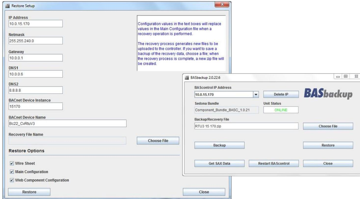
*Pre-built applications are provided in a BASbackup compatible zip file. Once the application is loaded, possibly modified, and then configured, the resulting version can be completely backed up using BASbackup thereby providing a comprehensive archive of the project. The proven version can then be used in cloning additional controllers only requiring a modification to individual IP addresses and BACnet device instances.*
