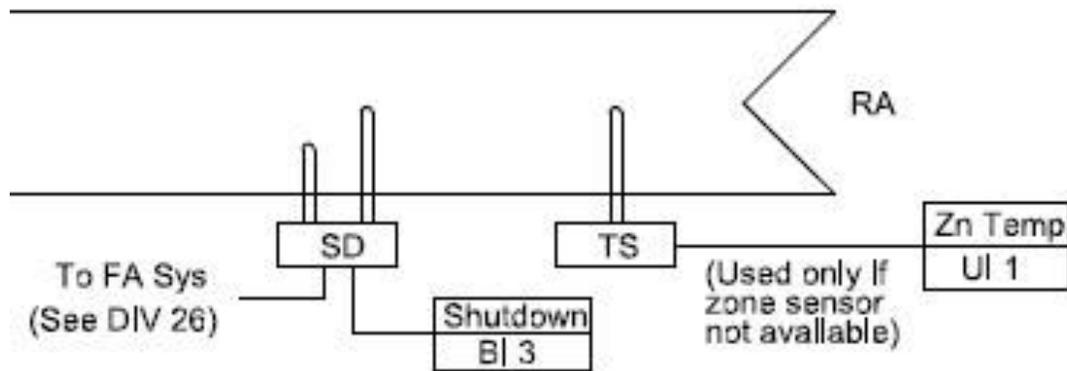
*For return air, you have a provision for a return air temperature sensor (TS) that can be in the return air duct or you can use a space temperature sensor that is mounted in the wall setter. A shutdown provision such as a smoke detector (SD) is provided to meet local fire code requirements.*
