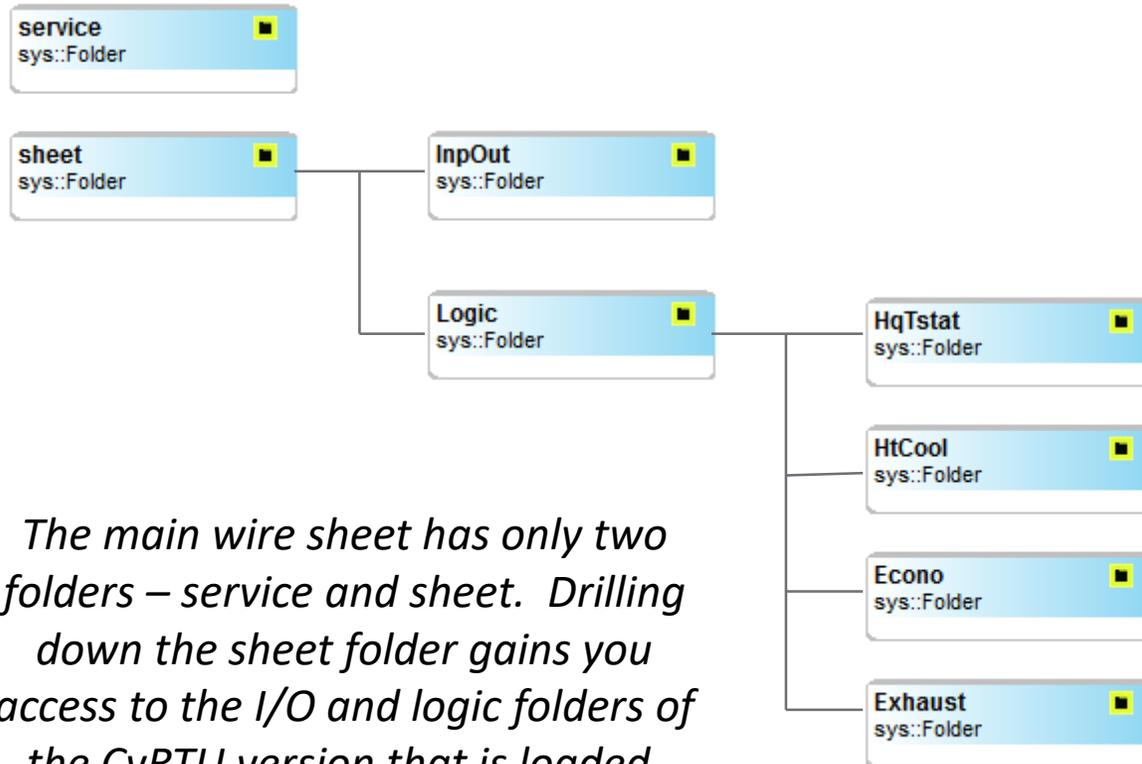
*The main wire sheet has only two folders – service and sheet. Drilling down the sheet folder gains you access to the I/O and logic folders of the CvRTU version that is loaded.*
