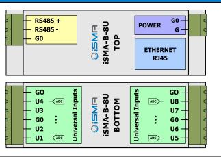
All G0 terminals are connected together internally
