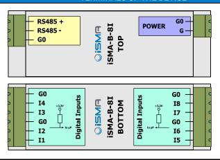
All G0 terminals are connected together internally
