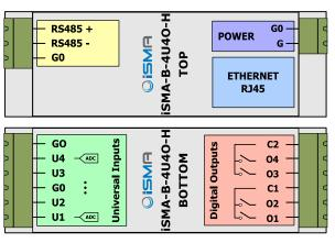
All GO terminals are connected together internally
