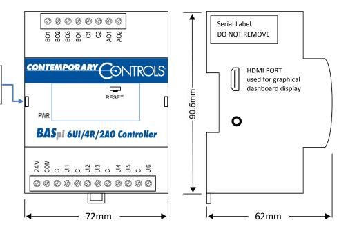
NOTE: Serial label covers the micro USB port which cannot be used to power the BASpi-Edge. Do not remove the serial label or BASpi-Edge warranty will be voided.
