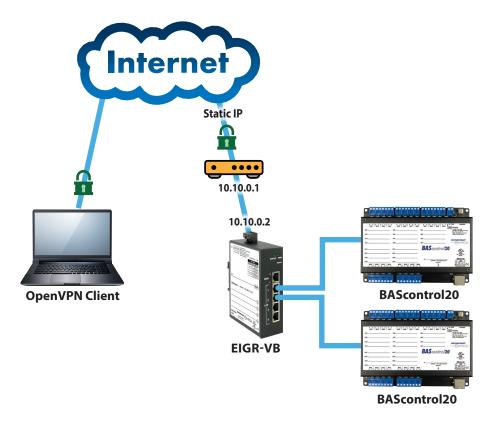
In the example above, if UDP port 5845 is being used as the OpenVPN port, the enterprise router/firewall at 10.10.0.1 will have a Port Forward entry for UDP port 5845 going to the VPN router at 10.10.0.2 at UDP port 5845. The EIGR-VB will use the Static IP of the enterprise router for OpenVPN configuration setup webpage.
