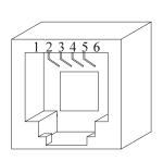
Figure 3 — Modular Jack Numbering Orientation
