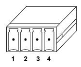
Figure 4 — Screw Terminal Connector Numbering Orientation
