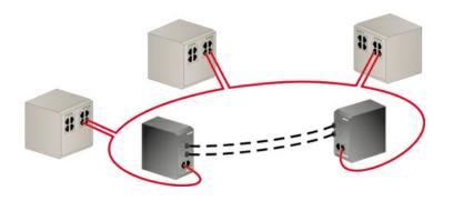
Media converters operating in transparency mode will faithfully carry critical link status in cable redundancy applications.
