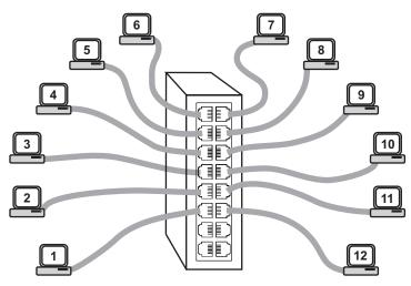
Figure 2. Wire-speed can be achieved if all stations are connected to a single switch.
