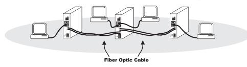
Figure 3. Mid-span switches require two backbone ports while end of line switches only require one. In this example, fiber optics are used for the backbone.
