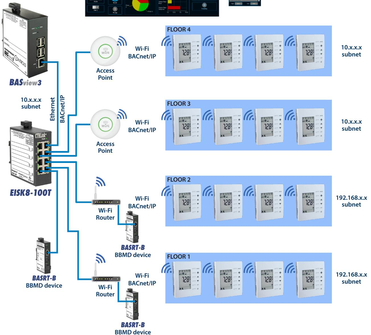
NOTE: Using a Wi-Fi router creates an additional subnet between the wireless network and the wired Ethernet. As is usual for any BACnet communication over subnets, BBMD devices are required on each subnet. BBMDs are not required if a Wi-Fi Access Point, that extends the same subnet as the wired Ethernet, is used to integrate the wireless thermostats.
