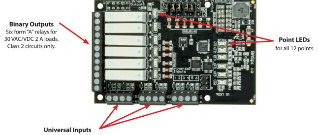
Six input channels can be configured — all discoverable as BACnet objects.
