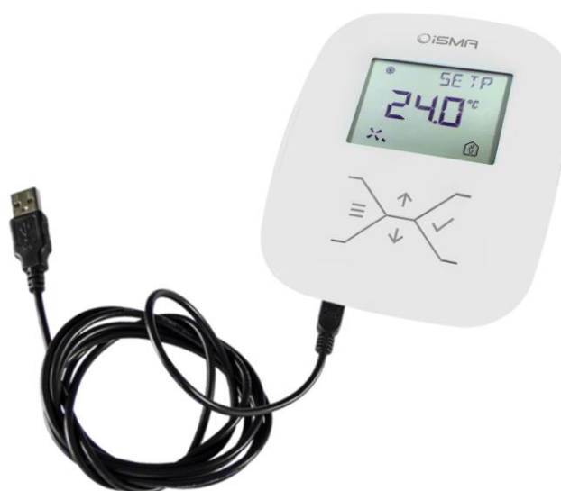
Figure 7 - Direct connection to iSMA-B-LP panel
