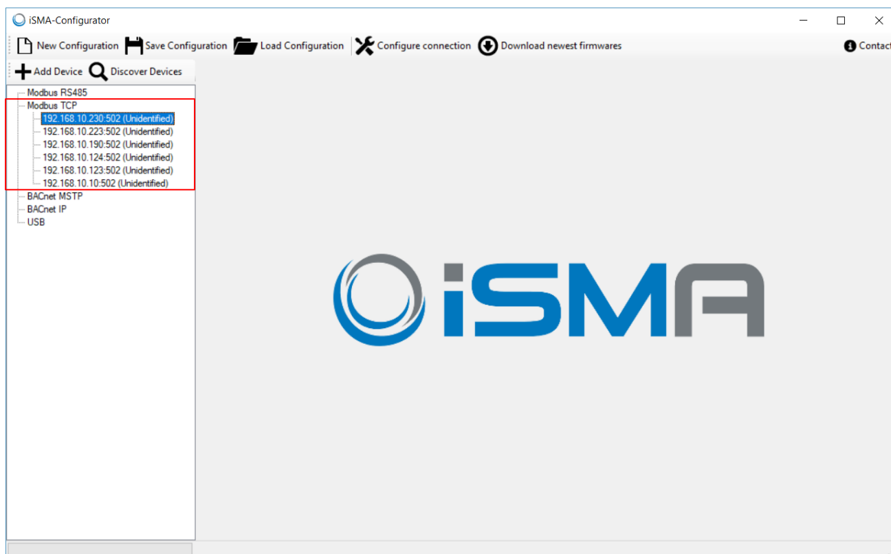
Figure 23 - Devices discovered via Modbus TCP
