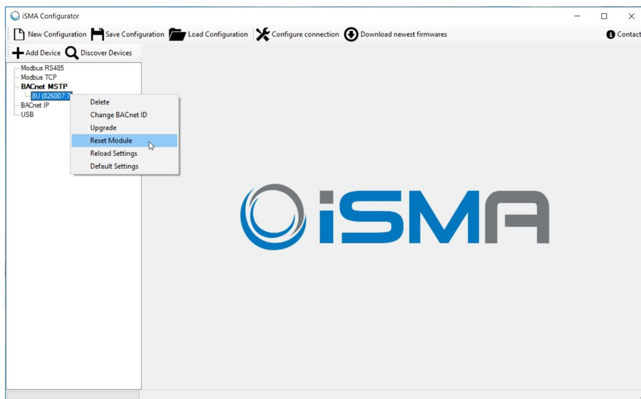
Figure 11 – Resetting the device
