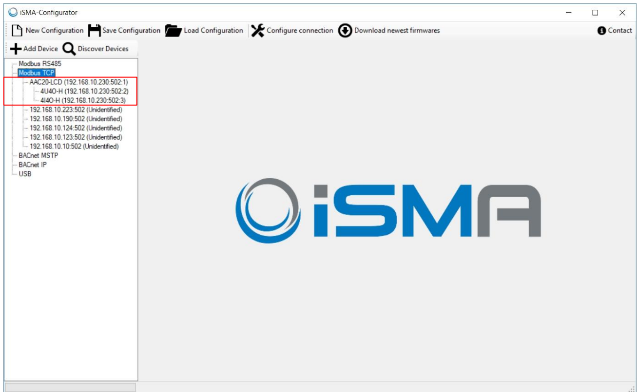
Figure 25 - Gateway devices discovered via Modbus TCP
